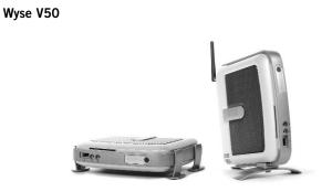
The high-performance Wyse V50 includes a powerful CPU; optional internal WiFi solution, optional smart card slot; CardBus/PCMCIA slot; plus serial, parallel, and USB ports. The Wyse V50 offers a broad range of mounting options via its innovative monorail mounting system that allows the unit to be conveniently attached to a wall, desk, or in any space-constrained environment.
