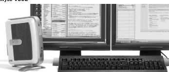
The mid-range Wyse V50L thin computer delivers the Linux performance you need; dual-video support (with purchase of optional monitor splitter cable); 128MB Flash, 256MB DDR RAM; a CardBus/PCMCIA slot; plus serial, parallel, and USB ports. Using the same form-factor as the Wyse V50, the Wyse V50L can fit easily into most work environments.
