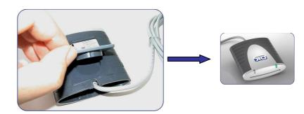
Or you can lift off the pad at the back of the reader so that it can be used without any base.
