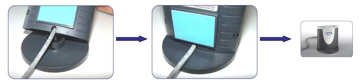
Pull the cable through the cut-out in the back of the reader.
